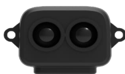
Figure 2 TF-LUNA Micro LiDAR.
