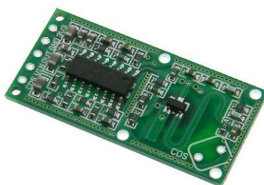
Figure 4 RCWL-0516 Microwave Radar.
