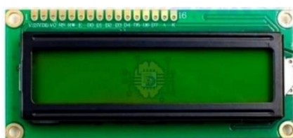
Figure 5 16x2 (1602) LCD Display.
